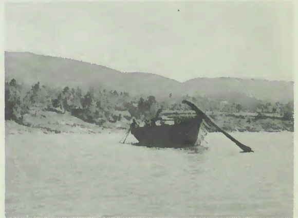
RABAO SHOWING STEERING OAR RABÃO MOSTRANDO O REMO-LEME
